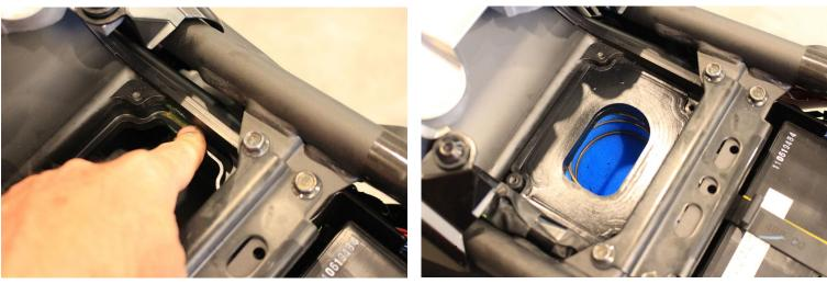
Grease the bottom sealing edge of the air box before placing the filter into position.
